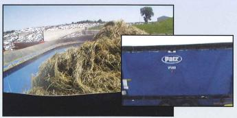
**Hay Retainer** chain is 5/16'' and hangs inside the top ring of the tub preventing the bale core from pushing hay out of the mixer.
