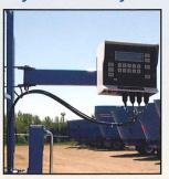
All scales are four-point mounted for load stability and accuracy of  $\pm$  .5% of system.
