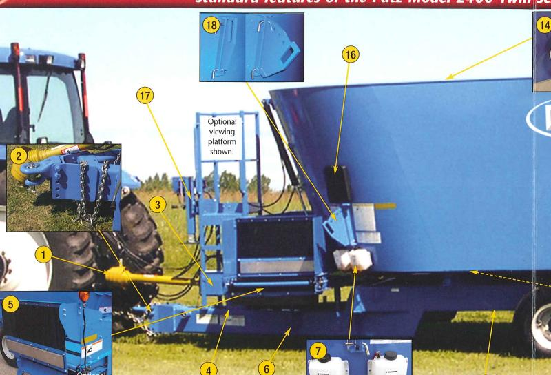
8" x 4" x 1/4" underslung "A" frame (over/under) design provides 18" of support at the point where forces are greatest and allows for a shorter turning radius. This frame design gives added strength in load carrying capacity and load turning strength.
